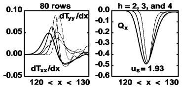
FIG. 9: The temperature gradients (the dashed lines correspond to the transverse temperature) for three values of h correspond to the heat fluxes found with the same h values. The pronounced maximum in  $T_{xx}$  indicates a violation of Fourier's Law, as the heat flux does not show a corresponding change of sign. The maxima in  $dT_{xx}/dx$  occur at distances 124.8, 124.3, and 123.8, significantly leading the flux maxima at 125.4, 125.3, and 125.2 for h = 2, 3, and 4.
