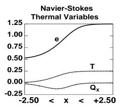
FIG. 3: The energy, (scalar) temperature, and heat flux vector from the Navier-Stokes equations are shown here. The heat conductivity and shear viscosity coefficients were assumed equal to unity in the underlying calculation.
