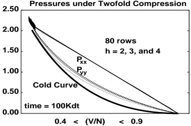
FIG. 7: Typical snapshot of the dependence of  $P_{xx}$  and  $P_{yy}$  on the volume (V/N). The line width increases with the range h = 2, 3, and 4. The range-dependence of  $P_{xx}$  is too small to be seen here while it is possible to see a small increase in  $P_{yy}$  with increasing h.
