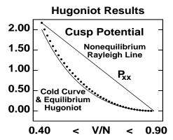
FIG. 4: The longitudinal pressure tensor component  $P_{xx}$  varies linearly with volume, and follows the Rayleigh line. The cold curve corresponds to the pressure of a perfect static triangular lattice. The equilibrium Hugoniot, indicated by dots, corresponds to thermodynamic equilibrium states accessible from the initial cold state by shockwave compression. For  $P_{yy}$  see Figure 7.
