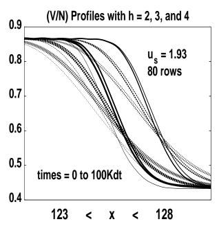
FIG. 5: Shockwave profiles at five equally-spaced times. The five line widths correspond to times of 0, 25,000dt, 50,0000dt, 75,000dt, and 100,000dt. The steepest profiles correspond to h=2. Results for h=3 and h=4 are also shown. The fourth-order Runge-Kutta timestep, here and throughout, is given by  $dt=0.02/u_s\simeq 0.01$ .
