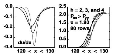
FIG. 8: The velocity gradient, for three values of h, is much more sensitive than is the shear stress,  $(P_{yy} - P_{xx})/2$ , to h. The gradient extrema, at 125.0, 124.65, and 124.3 precede the shear stress extrema at 125.67, 125.61, and 125.57 for h = 2, 3, and 4.
