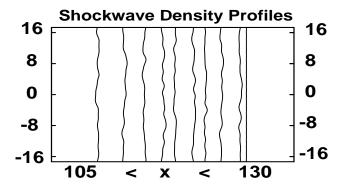
FIG. 6: Ten average-density contours (corresponding to the shockfront position) at equally-spaced times for a 40-row system. The amplitude of the fluctuations, of order unity, is similar to the range of the weight function h. The total timespan is 225,000 timesteps. Because the entrance velocity, at x = 0, is  $u_s = 1.92$ , rather than 1.93, the shockfront moves slowly toward the left, with a picture-frame velocity of about -0.01.
