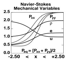
FIG. 2: The nonzero pressure-tensor components from the Navier-Stokes equations solution,  $P_{xx}$  and  $P_{yy}$ , as well as their average,  $P = (\rho^2/2) + \rho T$ , are shown as dashed lines along with the velocity, energy, and density profiles. In this simple example it is assumed that the bulk viscosity vanishes so that the average of the longitudinal and transverse components is equal to the equilibrium pressure.
