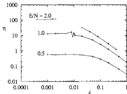
FIG. 2. Shear viscosity  $\eta \equiv -P_{xy}/\dot{\epsilon}$  for the Lucy potential with  $h=3\sqrt{m/\rho_0}$  and  $\rho=\rho_0$ . In order to make the present data comparable to those of Ref. [14], the strain rate and the shear viscosity from Table I, for  $h=6\sqrt{m/\rho_0}$ , have both been increased, by a factor 4.
