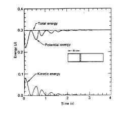
Fig. 10. Energy partition as a function of time. m =0.1 kg,  $\eta_0 = 0.2$  kPa sec,  $\alpha = 0.8$ .
