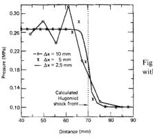
Fig. 15. Pressure profile within the shock front.
