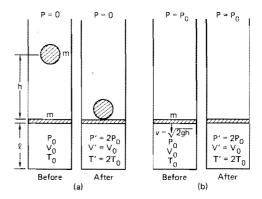
Fig. 1. Schematic diagram for problem I. (a) Exact treatment includes elastic bouncing of the weight on the piston. (b) Weight-piston interactions replaced by an averaged downward pressure  $P_0$ .
