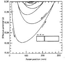
Fig. 12. Effective potential for piston motion.
