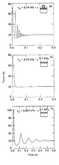
Fig. 2. Force-time history on the confining piston. (a) Calculation includes bouncing of the weight on the piston. (b) and (c) Weight-piston interaction replaced by an average downward pressure of 0.1 MPa.
