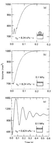
Fig. 4. Volume-time history. (a) Calculation includes bouncing of the weight on the piston. (b) and (c) Weightpiston interactions replaced by an average downward pressure of 0.1 MPa.
