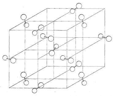
FIG. 2. Assumed crystal structure of the molecular solid, the so-called " $\alpha$ -nitrogen" structure. There are four molecules in the unit cell. The molecular axes lie parallel to the body diagonals of a cube.
