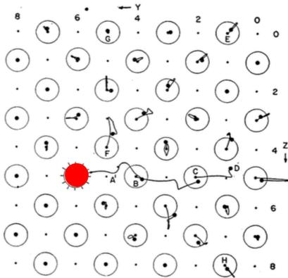
FIG. 6. Atomic orbits produced by shot in (100) plane at 40 ev.
