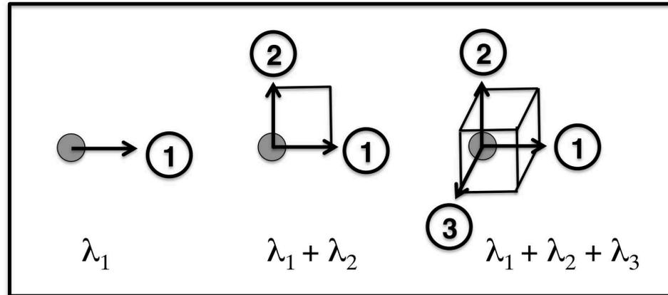
By following the motion of **N satellite systems** orthonormally constrained about an **N-dimensional reference system**, the **N Lyapunov exponents** are given by forces needed to maintain orthonormality. The algorithm was developed by Benettin's group.
