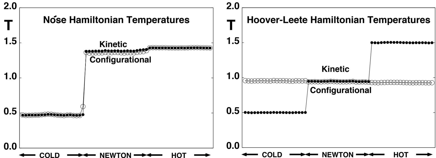
Despite tremendous temperature gradients there is **no heat flow** in these 60-particle  $\phi^4$  chains. The results are similar for the canonical and the kinetic thermostats. The interparticle forces are harmonic, with quartic tethers.
